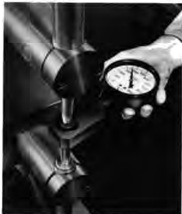
Large force gauge with maximum reading of 10,000 lb. Item No. 601-8100
